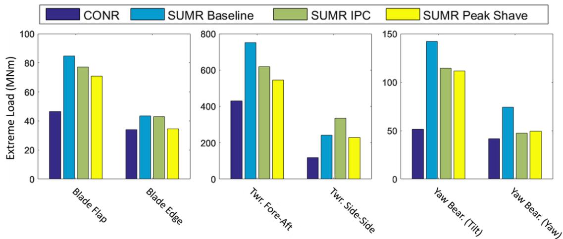
Figure 1. Extreme structural loads simulated for all power producing DLCs (1.1-1.5) for a conventional 13 MW rotor (dark blue), the SUMR with a baseline controller (light blue), the SUMR with individual pitch control (IPC) (green), and the SUMR with IPC and peak shaving (yellow).
