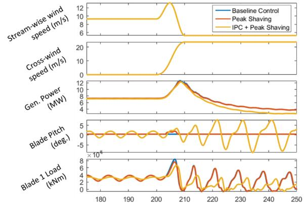
Figure 2. Extreme coherent ion change (DLC 1.4) at 2 m/s below rated; the load case with the greatest blade load. Wind speed, control signals and load simulations are shown for the SUMR rotor with baseline control (blue), peak shaving control only (red), and IPC with peak shaving control (yellow).
