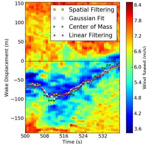
Figure 1: A comparison of methods is shown plotted against the flow field from SOWFA. The flow field is generated using a bilinear interpolation of SOWFA data at 6D downwind to enable equally spaced plotting.
