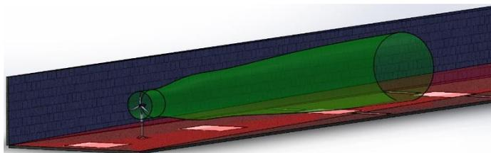
Figure 1 - Visualization of Turbine Wake and Boundary Layer Growth in UNH Flow Physics Facility.
