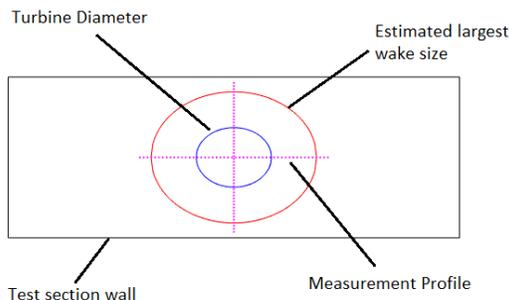
Figure 2 - Diagram of Pitot Tube Measurements. The “largest wake size” was estimated at 20 turbine diameters downstream of rotor plane based on previous measurements [2].
