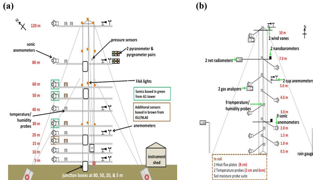
Fig. (a) A-tower instrument configuration for FaNTASTIC; (b) B-tower instrumentation
