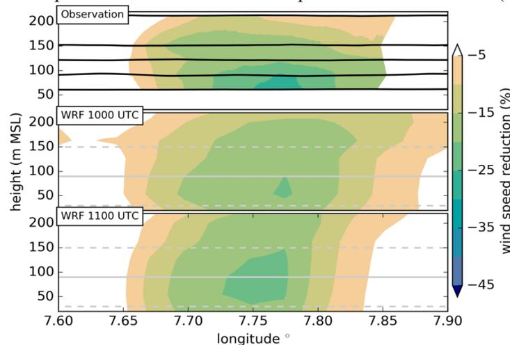
Figure 1: A comparison of observed and simulated wind speed reduction (colored contours) in a cross section perpendicular to the main flow, 5 km downstream of the wind farm clusters. The track of the air plane is indicated by black solid lines in the top panel. In the simulation panels the rotor area is indicated by a grey dashed line and the hub height by a solid grey line.
