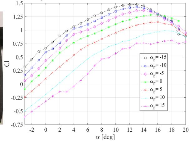
**Figure 2**  $C_1$  versus  $\alpha$  for different flap angles (simulation results)
