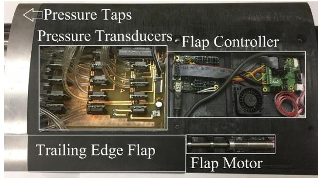
**Figure 1** In-blade surface pressure measurements and flap actuation and control
