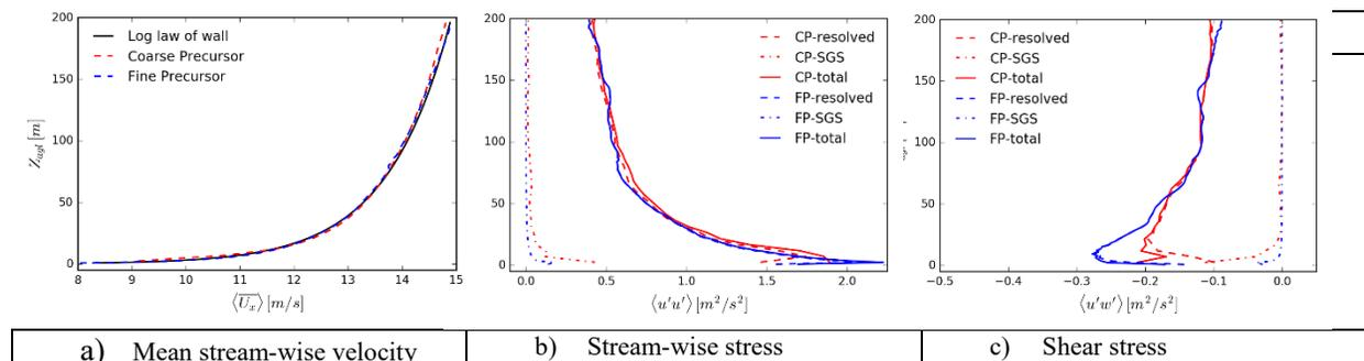
Figure 1: Comparison of wind velocity and stresses between coarse and fine precursor LES.
