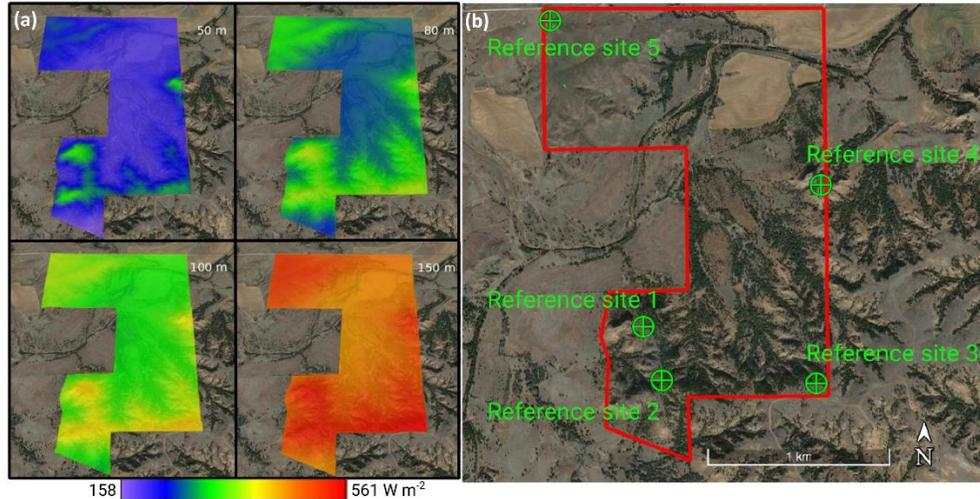
Figure 1. (a) Wind power density maps. (b) Five best sites for wind turbine installation.
