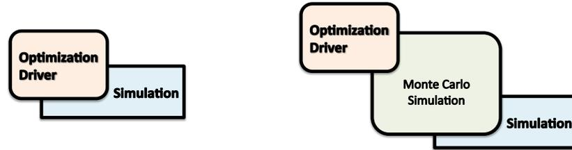
Figure 1: Classically, an optimizer deterministically optimizes a model (left). In OUU (right), an uncertainty quantification routine is used to simulate several possible scenarios. Statistics describing those scenarios are optimized.
