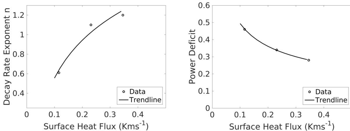
**Figure 1:** a) Decay Rate Exponent for single wind turbine wakes. b) Power Deficits for Aligned Wind Turbine 4D downstream. c) Decay Rate Exponent for Downstream Wind Turbine Wakes Aligned 4D downstream.
