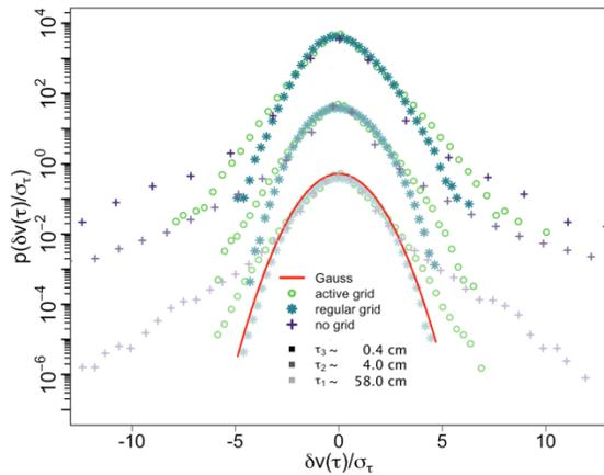
**Figure 1** Increment PDFs for the different inflow condition measured at rotor plane – the time scales correspond to rotor-related scales ( $\tau_1 \sim D$ ,  $\tau_2 \sim$  chord length,  $\tau_3 \sim$  chord thickness); the PDFs are shifted vertically for clarification
