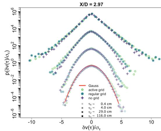
**Figure 2** comparison of increment PDFs in the wake for different inflow conditions at 2.97D distance plane – the time scales correspond to rotor-related scales ( $\tau_1 \sim 2D$ ,  $\tau_2 \sim D/2$ ,  $\tau_3 \sim$  chord length,  $\tau_4 \sim$  chord thickness); the PDFs are shifted vertically for clarification
