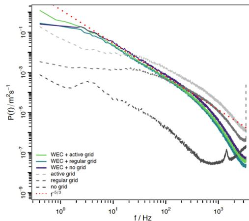
**Figure 3** Comparison of the power spectra of the different inflow conditions measured at rotor plane (grey) with the power spectra at 2.97D distance in the wake for the respective inflows
