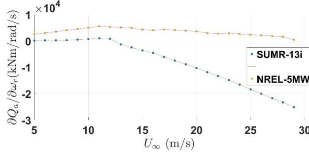
Figure 1-Aerodynamic torque sensitivity with respect to rotor angular velocity as a function of wind speed
