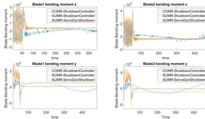
Figure 2. Blade bending moments before and after shutdown
