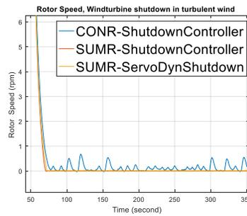
Figure 1. Rotor speed comparison before and after shutdown
