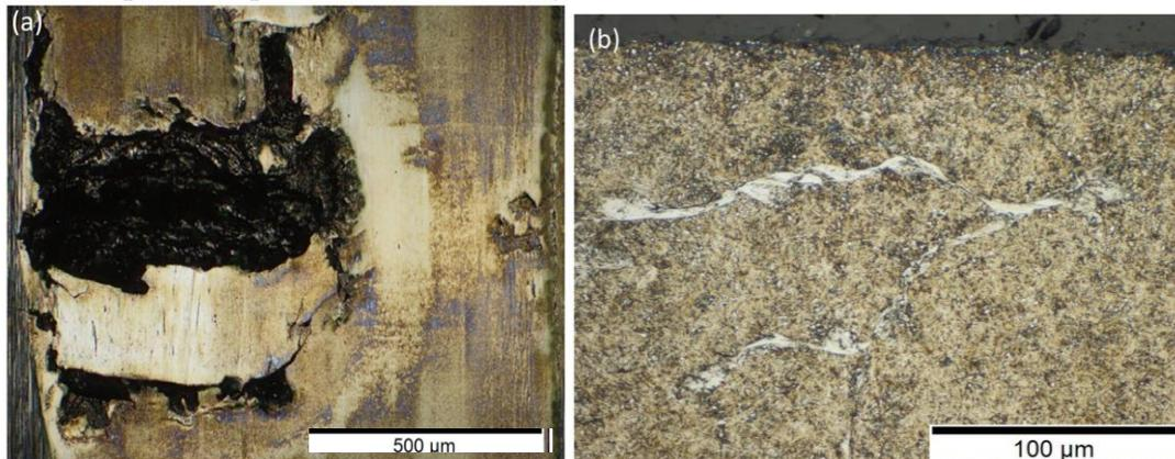
**Figure 2. View of roller race spall (left) and cross section with WECs (right) [3]**
