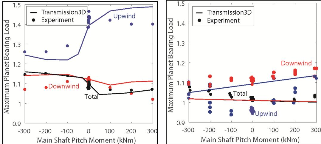
**Figure 1. Maximum planet bearing loads in CRBs (left) and TRBs (right) [2]**
