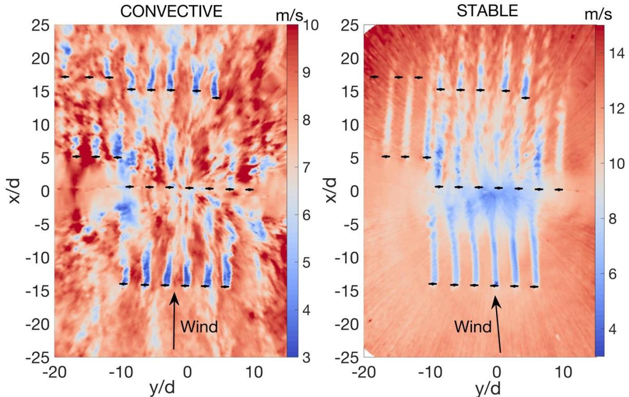
Figure 1: Horizontal equivalent velocity measured with a scanning LiDAR with the PPI technique over a conical surface with elevation angle of  $3^\circ$ . Measurements are carried out under different atmospheric stability regimes: (lhs) convective; (rhs) stable.
