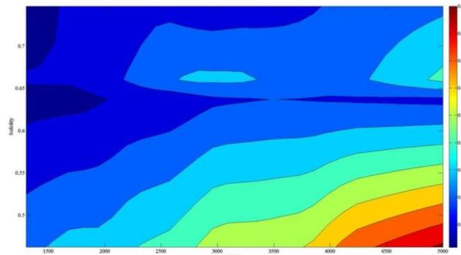
Figure 2 Swirl Strength Contour at 30 m/s
