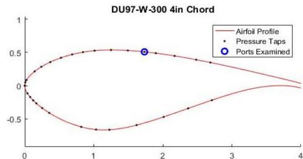
Figure 1: DU97-W-300 Wind Turbine airfoil geometry. Pressure Tap locations are listed as black points, and the blue circle pinpoints the port examined in the results section.
