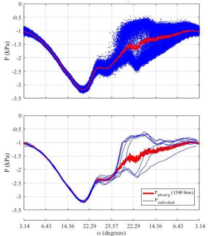
Figure 2: for the DU97-W-300 airfoil,  $14^\circ \pm 10^\circ$ ,  $x/c = 0.4332$  (top): (a) All pressure data with Phase Averaged data for reference. (b) Averaged data compared with data from eight arbitrary pitch cycles.
