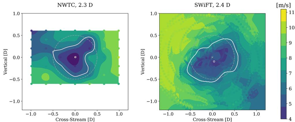
Fig. 1: Example wake measurements at NWTC (2.3 D downstream of wind turbine) and at SWiFT (2.4 D downstream of wind turbine). Data are snapshots, and contour values are consistent for both plots. Dashed gray line indicates rotor area and gray marker the hub location. White solid line indicates wake outline and white circle its center.
