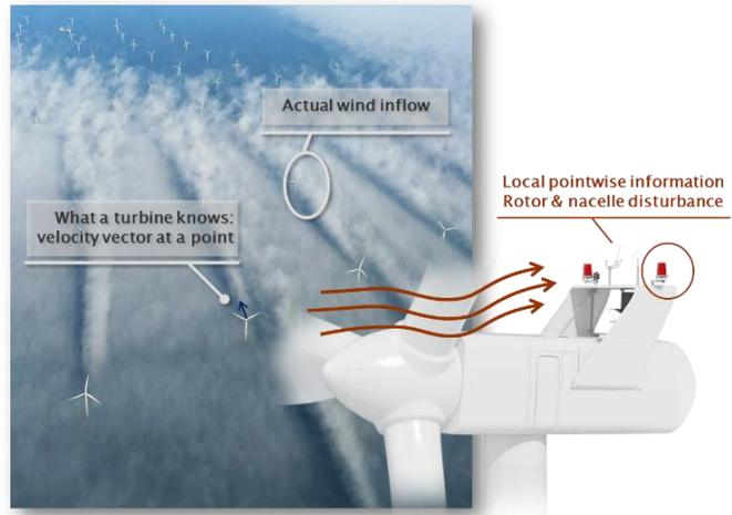
Figure 1. The limited knowledge of wind conditions available to a wind turbine today, compared to the actual complexity of the inflow.
