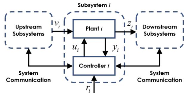
Figure 1- LC-DMPC system structure, figure adapted from [3].
