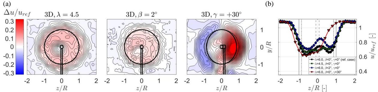
Figure 1: (a) Added mean velocity  $\Delta u/u_{ref}$  in the wake  $x/D=3$  downstream of the turbine T1 by  $\lambda$ -control,  $\beta$ -control and  $\gamma$ -control of the upstream turbine. (b) Mean velocity profiles  $u/u_{ref}$  at the turbine hub height at  $x/D=3$ . The inflow is uniform ( $TI_B=10.0\%$ ).
