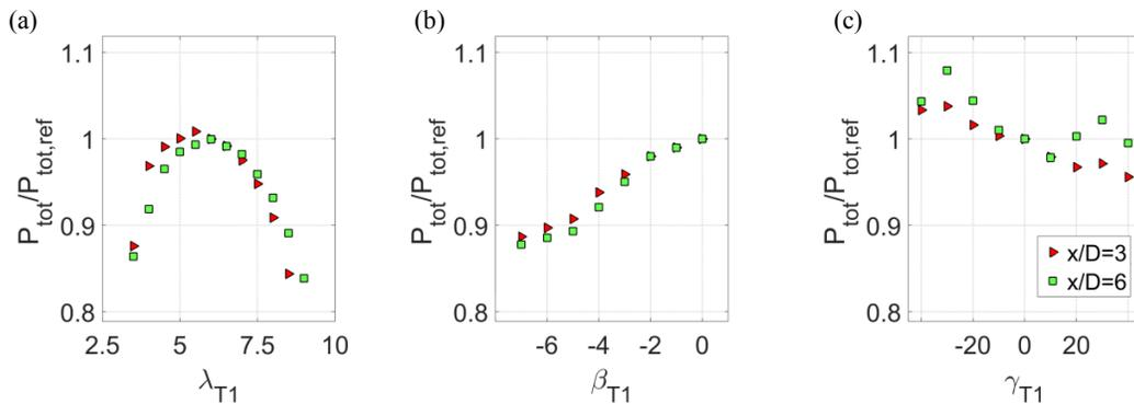
Figure 2: Relative total power of the two-turbine array for (a)  $\lambda$ -control (b)  $\beta$ -control and (c)  $\gamma$ -control of the upstream turbine. The separation distance is  $x/D=3$  respectively  $x/D=6$ . The inflow is uniform ( $TI_B=10.0\%$ ).
