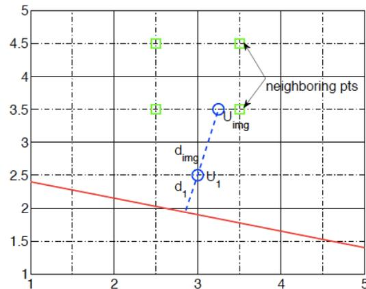
Figure 1. Schematic of velocity reconstruction log-law immersed boundary method.
