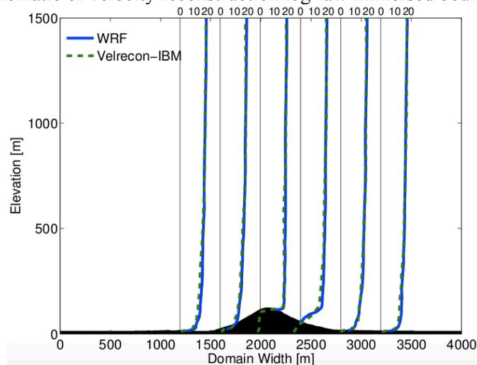
Figure 2. Wind profiles over Askervein Hill for WRF and WRF-IBM with velocity reconstruction.
