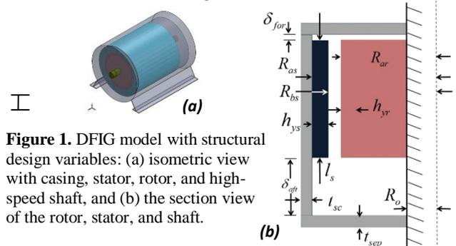
Figure 1. DFIG model with structural design variables: (a) isometric view with casing, stator, rotor, and high-speed shaft, and (b) the section view of the rotor, stator, and shaft.
