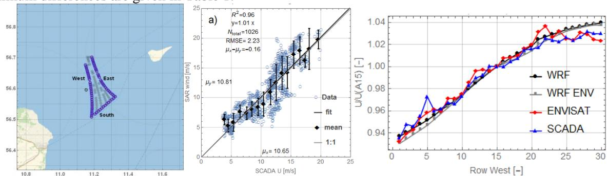
**Figure 1:** Left: Location of the wind turbines of the Anholt wind farm. In blue, turbines used for comparisons with SAR wind retrievals. Middle: Comparison of Sentinel-1 SAR and SCADA for turbines in the free stream for row west, south, and east. Right: SCADA, SAR and WRF wind speeds nondimensionalized with turbine number 15 for row West with wind directions between  $245^\circ$  and  $275^\circ$ . The turbines are numbered from South to North.
